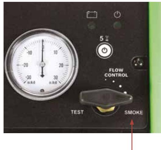
**FLOW CONTROL** controls smoke volume. Locating the leak source is sometimes even easier with less smoke volume exiting a leak. After filling a system with smoke in the SMOKE (full open) setting, use the smoke volume control knob to tune in the desired volume of smoke exiting a leak.
