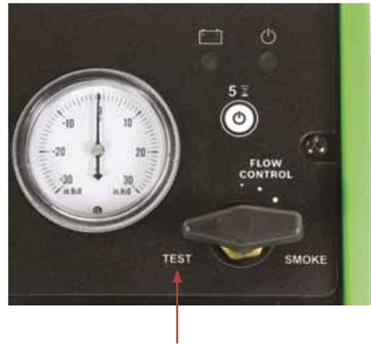
**SMOKE** (full open) setting delivers maximum smoke volume to the system being leak tested.
