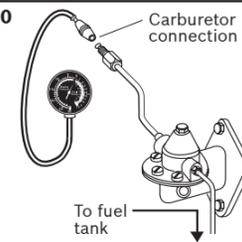
**NOTE:** The fuel in the carburetor fuel bowl will be sufficient to run the engine for these tests.
