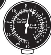
on non-emission controlled engines (pre-1968) indicates correct engine vacuum. Readings may vary considerably on different engines, but should not fall below these minimums. (See manufacturer's specifications).
