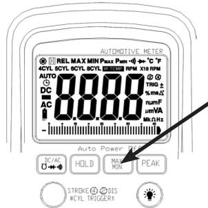
2. Press the **MAX/MIN** key and a blinking “**MAX MIN**” will appear. The meter will display the present reading, but will continue to update and store the max and min readings.
