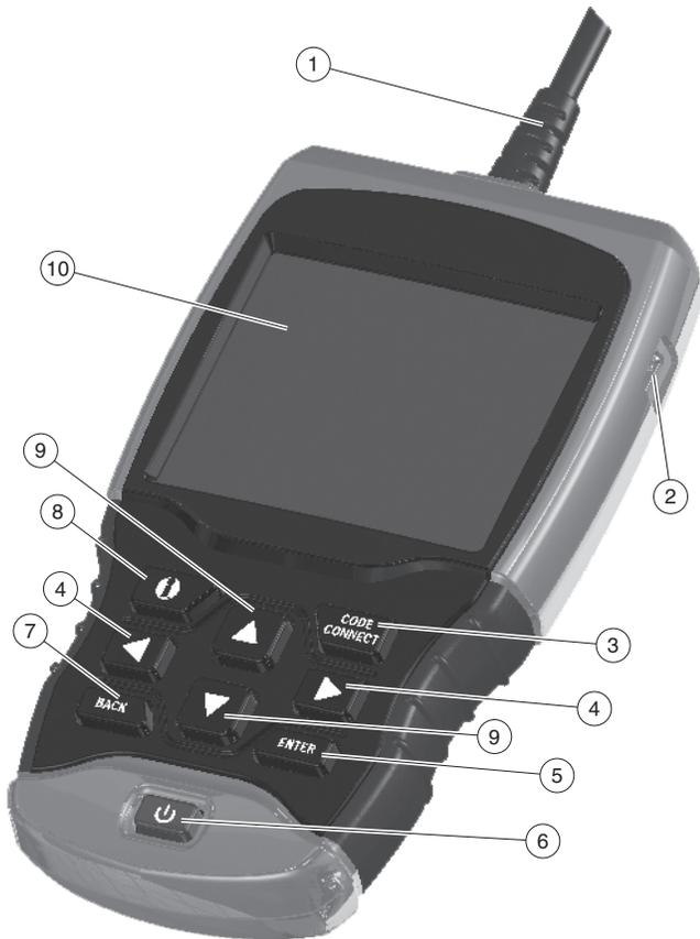
1. DLC Cable - provides connection for vehicle interface.
