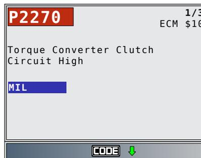
Pending indicates a global OBDII/EOBD pending code.
