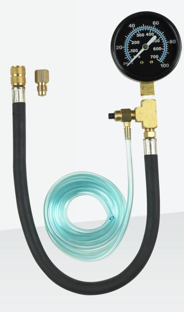
The Fuel Pressure Tester Kit works on most domestic fuel injected vehicles having a Schrader valve test port on the fuel rail. This includes Ford high pressure central fuel injection and GM, Ford, and Chrysler multi-port fuel injection. Multi-port means one fuel injector per cylinder.
