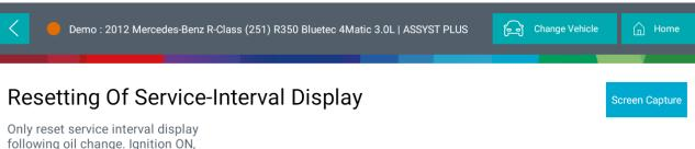
following oil change. Ignition ON, engine must not run.
