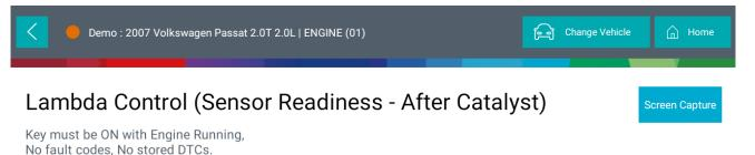
Lambda Control (Sensor Exchange) – Tests and compares Oxygen Sensors, after Catalytic Converter, to the Air Mass to make sure they are working properly
